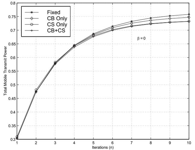
Fig. 7. Total Mobile Transmit Power in Uniform Azimuthal Traffic,  $\beta = 0$ .
