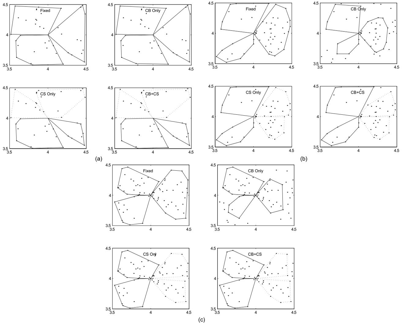
Fig. 3. Center cell coverage: (a) - with no hot-spot sector (uniform azimuthal traffic,  $\beta = 0$ ). (b) - with one hot-spot sector (nonuniform azimuthal traffic,  $\beta = 2$ ). (c) - with two hot-spot sectors (nonuniform azimuthal traffic,  $\beta = 2$ ).
