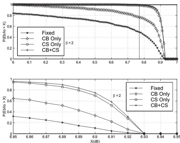
Fig. 9. Complementary CDF of received signal quality for all mobiles in nonuniform azimuthal traffic in the center cell,  $\beta = 2$ . A (randomized) single hot-spot sector is included.
