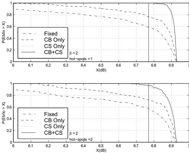
Fig. 10. Complementary CDF of received  $E_b/I_o$  for all users in nonuniform azimuthal traffic in the center cell,  $\beta = 2$  with one hot-spot (top graph) two hot-spots (bottom graph).
