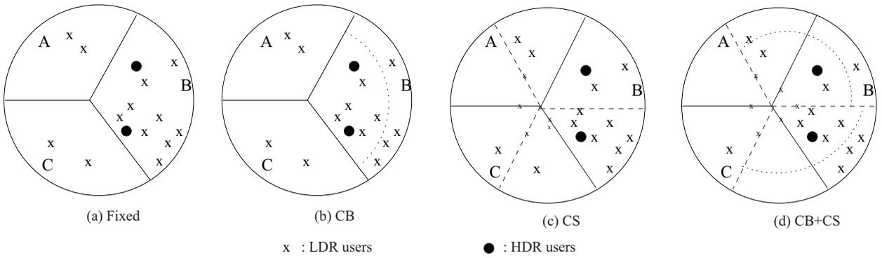
Fig. 2. Spatial interference control techniques. Low data rate (LDR) and high data rate (HDR) users co-exist in the system. In (c) and (d), dashed and solid lines denote the sectors of two different groups of non-overlapping sectors. Dotted lines denote the shrinking of the cell/sector size.
