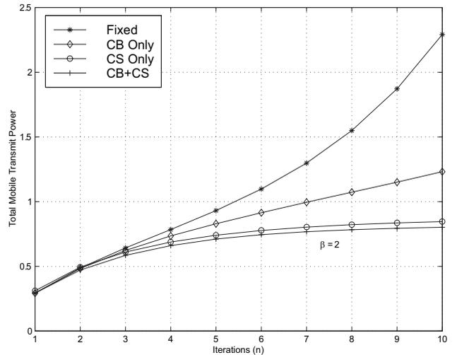
Fig. 8. Total Mobile Transmit Power in Nonuniform Azimuthal Traffic,  $\beta = 2$ .
