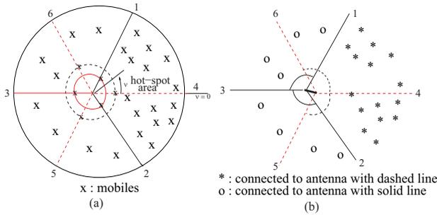
Fig. 5. An FOSAA [6,2] is implemented in a cell: (a) hot-spot area and (b) a hypothetical base station antenna assignment for mobiles.
