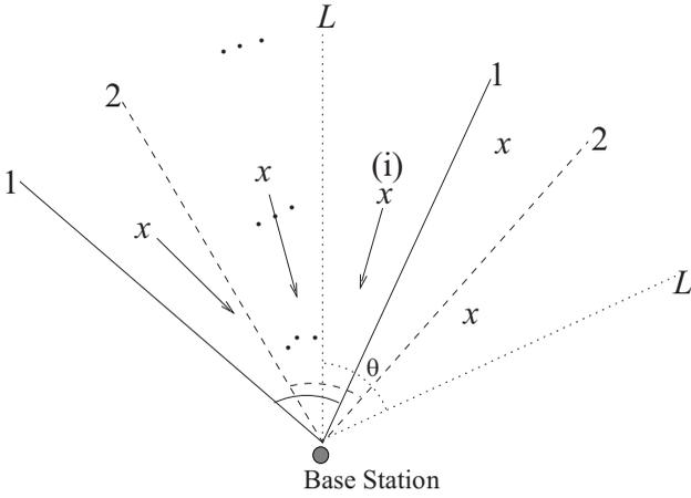
Fig. 1. Mobile  $i$  can potentially be covered by  $L$  antenna in FOSAA. Antenna "1" receives signals from users who may possibly be in communication with  $L$  different (co-located) antenna.
