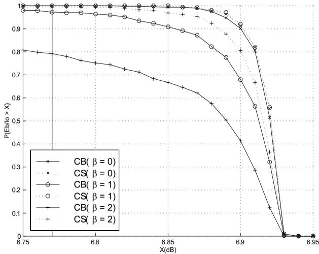
Fig. 6. Complementary CDF of  $E_b/I_o$  with sector congestion control parameter ( $\beta$ ). A (randomized) single hot-spot sector is included.
