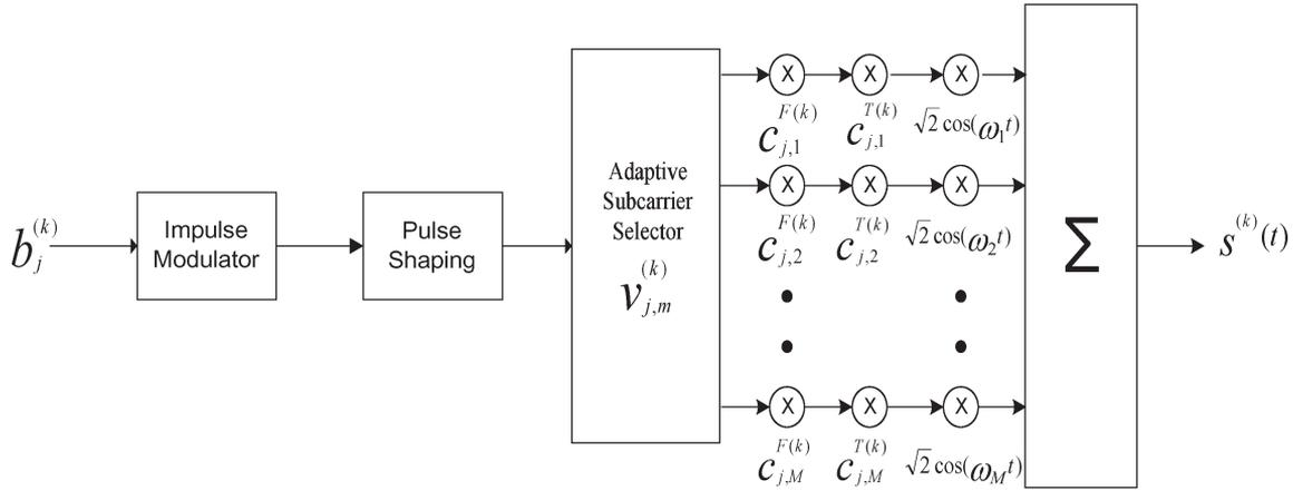
Fig. 2. Block diagram for the adaptive multicarrier CDMA system with time and frequency spreading.
