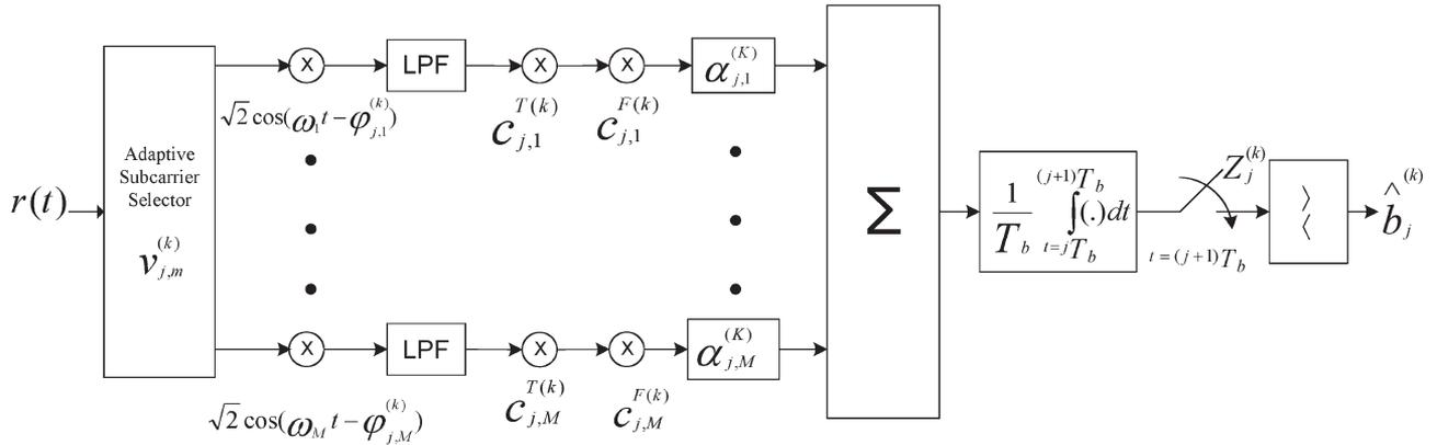
Fig. 3. Receiver block diagram for adaptive multicarrier CDMA system with time and frequency spreading.
