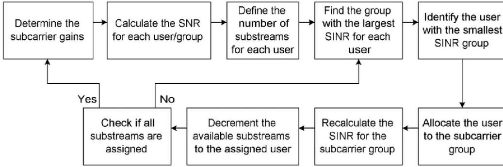
Fig. 4. Adaptive subcarrier allocation flowchart.
