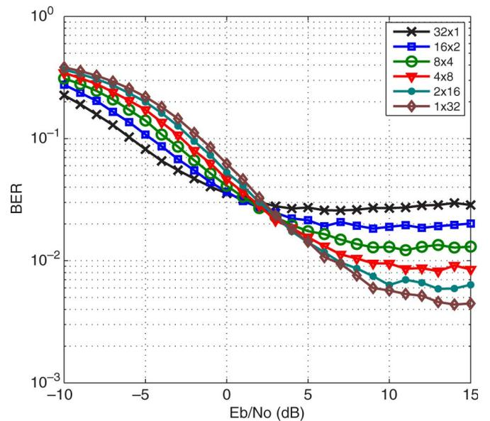
Fig. 6. BER versus  $E_b/N_o$  for adaptive multicarrier CDMA system with various spreading factors.
