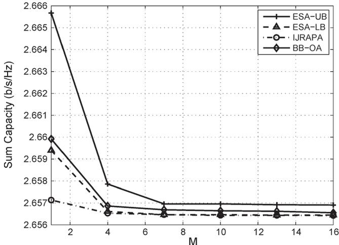
Fig. 5. Sum-rate capacity versus number of PUs. The parameters are  $L = 4$ ,  $K = 2$ ,  $I_m^{\max} = 1 \text{ mW}$ ,  $p_s^{\max} = 1 \text{ W}$ , and  $p_l^{\max} = 1 \text{ W}$ .
