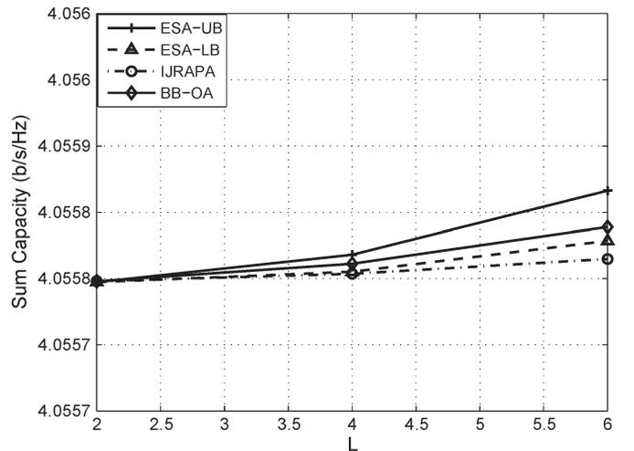
Fig. 4. Sum-rate capacity versus number of relays. The parameters are  $M = 16, K = 2, I_m^{\max} = 100 \mu\text{W}, p_s^{\max} = 1 \text{ W},$  and  $p_l^{\max} = 1 \text{ W}$ .
