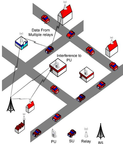
Fig. 1. Vehicular network with multiple relays.
