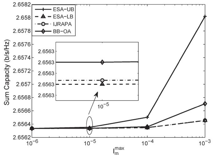
Fig. 3. Sum-rate capacity versus interference threshold (in watts). The parameters are  $L = 6, K = 2, M = 16, p_s^{\max} = 1 \text{ W},$  and  $p_l^{\max} = 1 \text{ W}$ .
