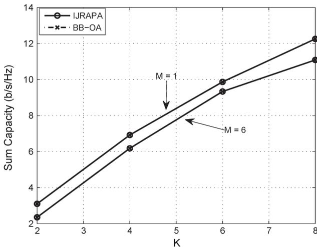
Fig. 6. Sum-rate capacity versus number of SUs. The parameters are  $L = 16$ ,  $I_m^{\max} = 1 \mu\text{W}$ ,  $p_s^{\max} = 1 \text{ W}$ , and  $p_l^{\max} = 1 \text{ W}$ .
