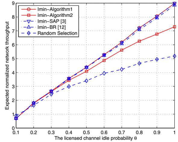
Fig. 8. Companion results for the simulated small network with Log-normal fading ( $P_t = 1W$ ,  $\beta = 2$  and  $\sigma_{dB} = 6dB$ ).
