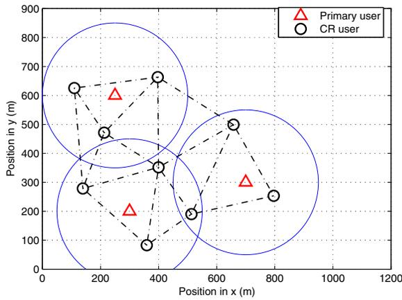
Fig. 3. The simulated small CRN. (Each circle represents a CR link, and the dashed lines represent the bilateral interferences between the CR users).
