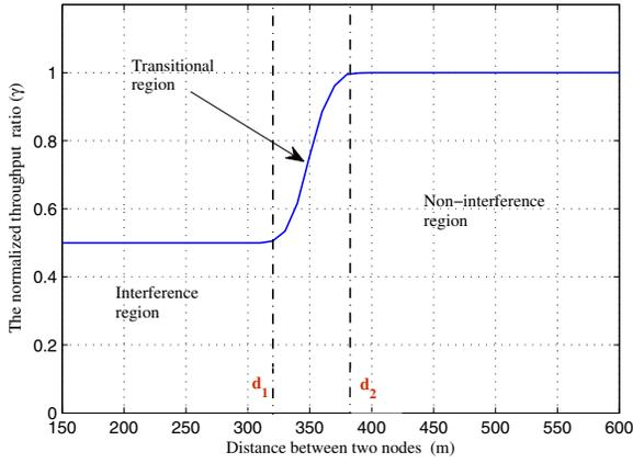
Fig. 1. The effect of mutual interference on the achievable throughput.
