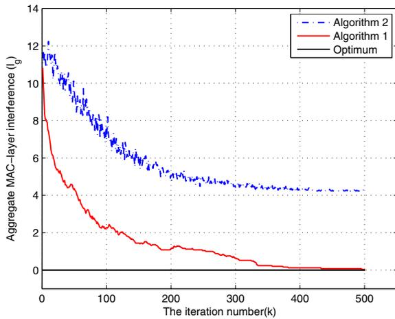
Fig. 4. The expected convergence behaviors of the two algorithms for the simulated CRN.
