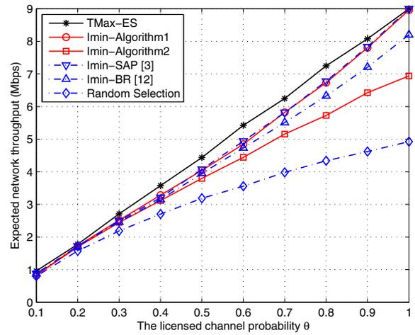
Fig. 5. Companion results of six channel selection methods for the simulated small network with no fading (For the learning algorithms, we set  $\beta = 10 + k/50$  for Algorithm 1 and  $b = 0.05$  for Algorithm 2).
