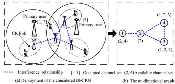
Fig. 2. An example of the considered BI-CRN with four licensed channels. Note that CR users 2 and 3 will interfere with each other when transmitting on the same channel, whereas user 1 will never interfere with user 3.
