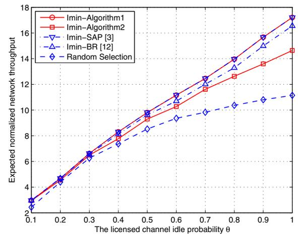
Fig. 9. Companion results for the simulated large network with Log-normal fading ( $P_t = 1W$ ,  $\beta = 2$  and  $\sigma_{dB} = 6dB$ ).
