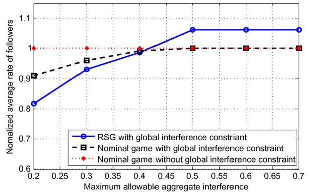
Fig. 8. Normalized average rate of followers under different level of aggregate interference constraints.
