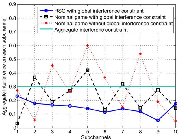
Fig. 11. The aggregate interference experienced by a user of an MBS under different solutions.
