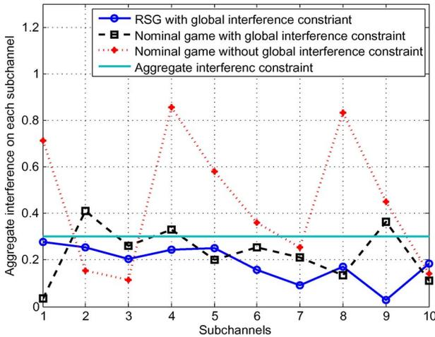
Fig. 10. The aggregate interference experienced by a user of an MBS under different solutions.
