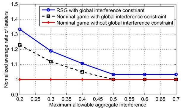
Fig. 9. Normalized average rate of leaders under different level of aggregate interference constraints.
