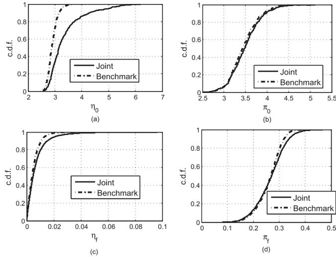
Fig. 6. The CDF of EE (a) and SE (b) for the MeNB, and the CDF of EE (c) and SE (d) for the SeNB.
