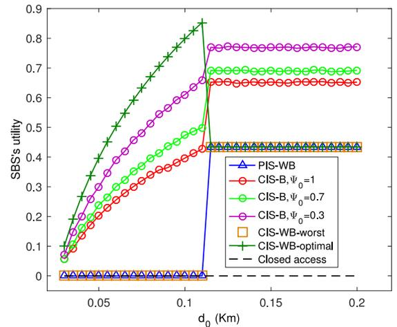
Fig. 5. SBS's utility versus the distance between MBS and MUE.
