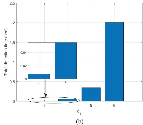
Fig. 7. Detection complexity experienced by SCMA receivers with  $d_c = 2$ . (a) Total operations required for SCMA detection. (b) Time required by an IoT device with 20 MHz processing capacity.
