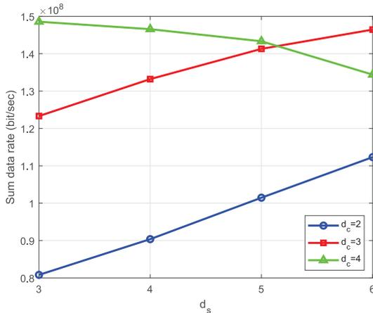
Fig. 4. Effect of  $d_s$  and  $d_c$  on the sum data rate.
