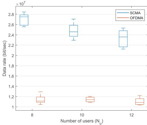
Fig. 6. Comparison of the per-user data rate between SCMA and OFDMA systems at  $N_u = 8, 10,$  and  $12$ .
