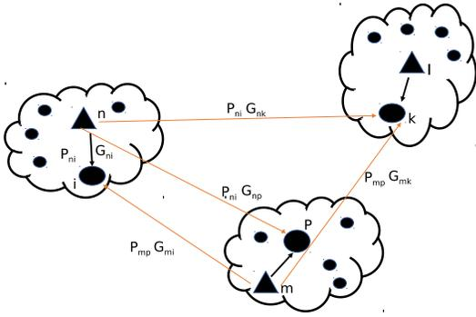
Fig. 3. Interference graph.
