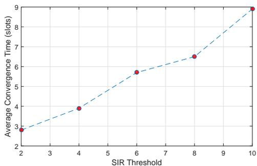
Fig. 11. Convergence time at various SIR thresholds
