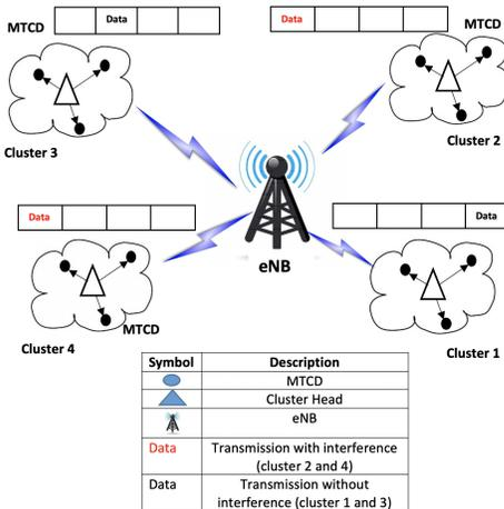
Fig. 1. Clustered IoT/M2M network.
