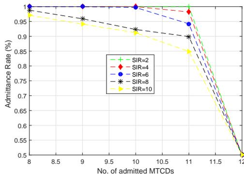
Fig. 13. Successful smart devices/MTCDS at various SIR thresholds
