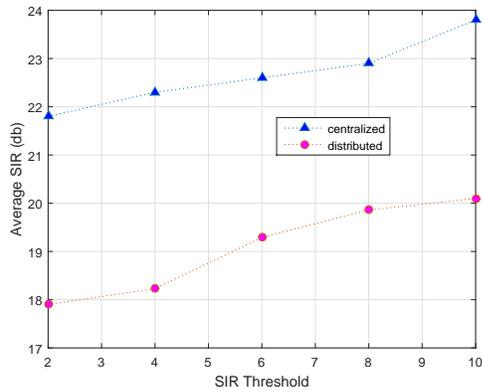
Fig. 8. Average SIR for centralized and distributed allocation
