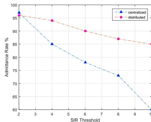
Fig. 7. Admittance rate for centralized and distributed allocation
