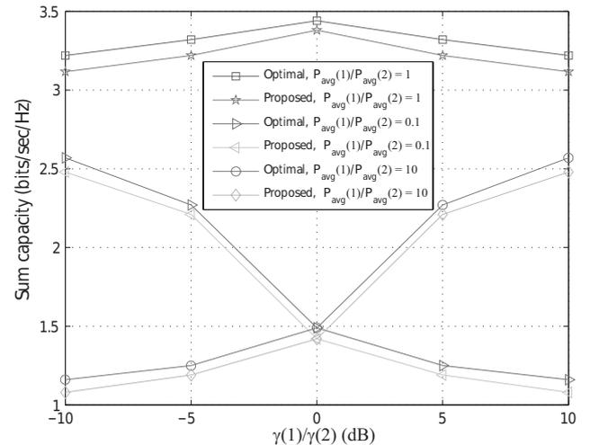
Fig. 10. Performance comparison of proposed scheme and optimal algorithms for the case of two users and ten subchannels.
