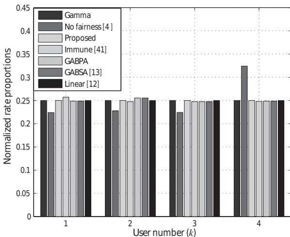
Fig. 8. Normalized capacity ratios per user for 4 users averaged over 100 channels, with the required normalized proportions  $\gamma$  shown as the leftmost bar for each user.
