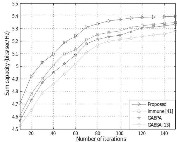
Fig. 5. Sum capacity versus number of iterations ( $K = 16$ ,  $N = 64$ ).
