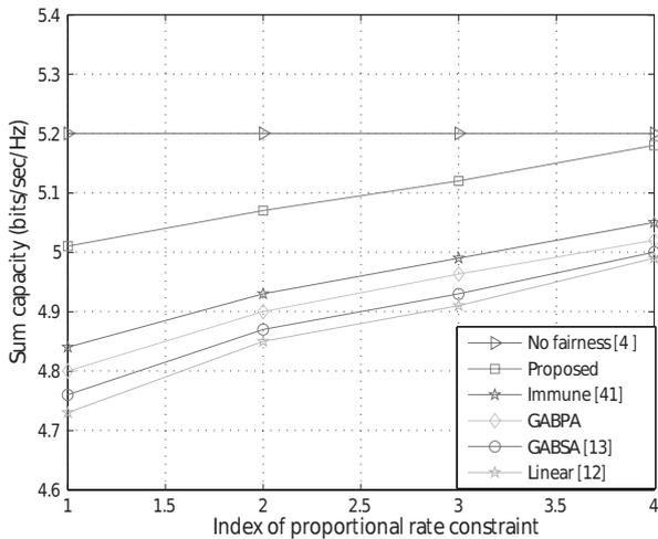
Fig. 7. Sum capacity versus index of proportional rate constraint (see Table 2 for index values).
