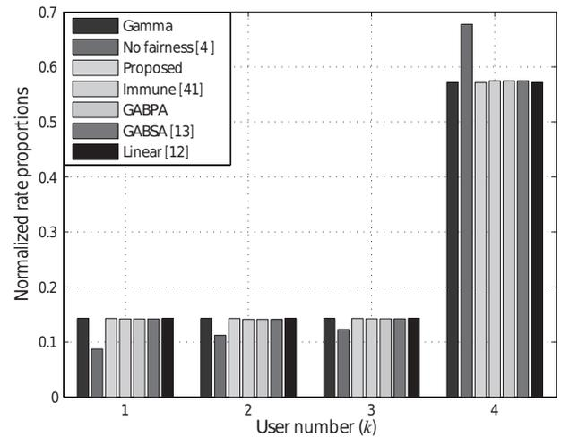
Fig. 9. Normalized capacity ratios per user for 4 users averaged over 100 channels, with the required normalized proportions  $\gamma$  shown as the leftmost bar for each user.
